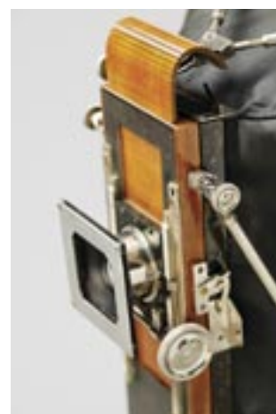
Survey camera built by Albrecht Meydenbauer, close-up of lens, 1898
