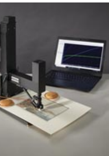
Using a microfade tester to determine how long an object can be exhibited for.
